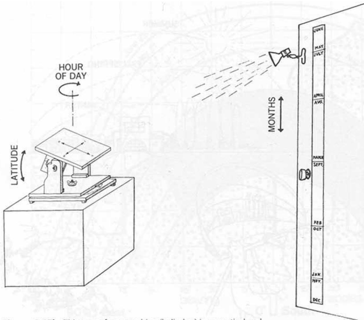
**Figure 6.15b** This type of sun machine (heliodon) is a practical and appropriate tool for every design studio.
