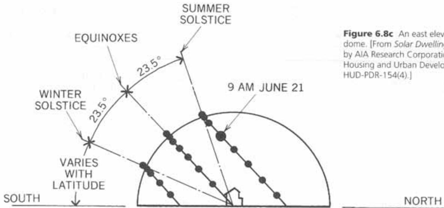
**Figure 6.8c** An east elevation of the sky dome. [From *Solar Dwelling Design Concepts* by AIA Research Corporation. U.S. Dept. Housing and Urban Development, 1976. HUD-PDR-154(4).]
