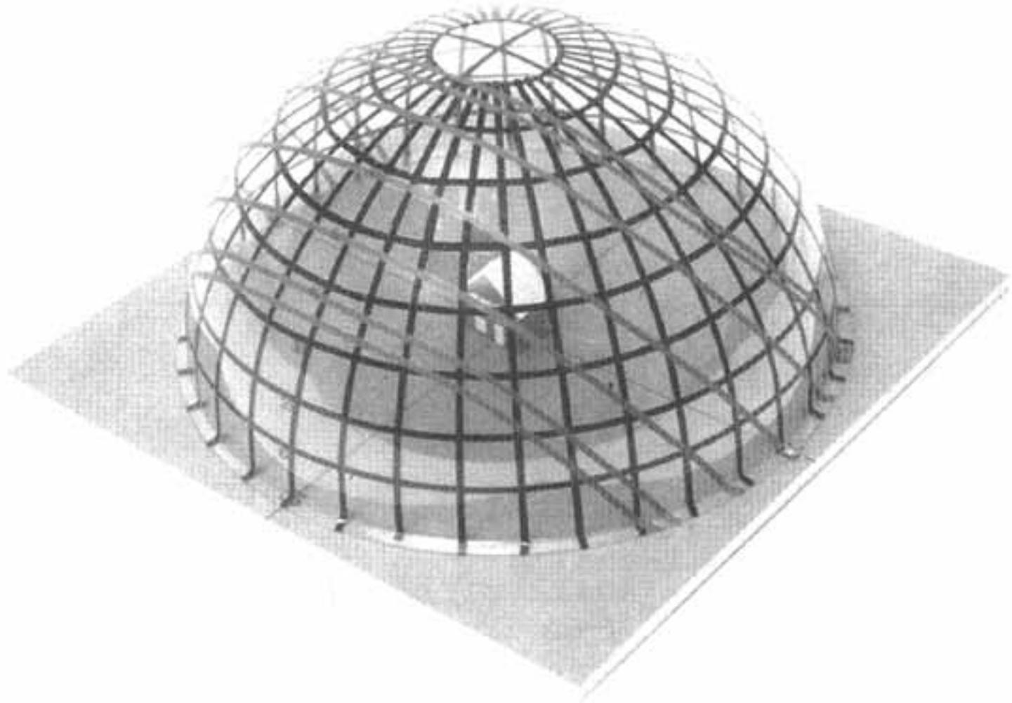
**Figure 6.11b** A model of the sky dome. The sun paths for the 21st day of each month are shown. Only seven paths are needed for twelve months because of symmetry (i.e., May 21 is the same path as July 21).
