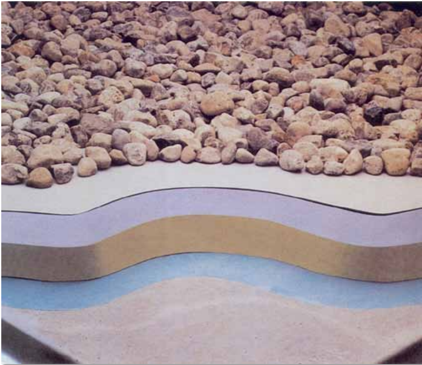
Loose laid, ballasted, membrane
