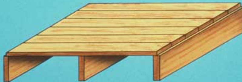
TWO SPAN CONTINUOUS PATTERN
