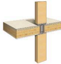
partial encapsulation during construction
