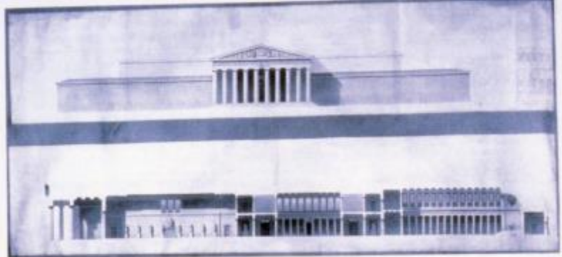
84, 85 H. Labrouste. Cour de Cassation, 1824: rendered elevation and longitudinal section (above), and rendered cross-section of main courtroom. (Deux-Arts)
