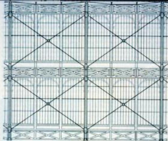
WROUGHT-IRON RODS provided a rigid support for the exterior walls of the Crystal Palace, which had no internal walls to stiffen it. Visible from inside and out (the interior view is shown here), these cross braces added to the building's strikingly contemporary appearance.
