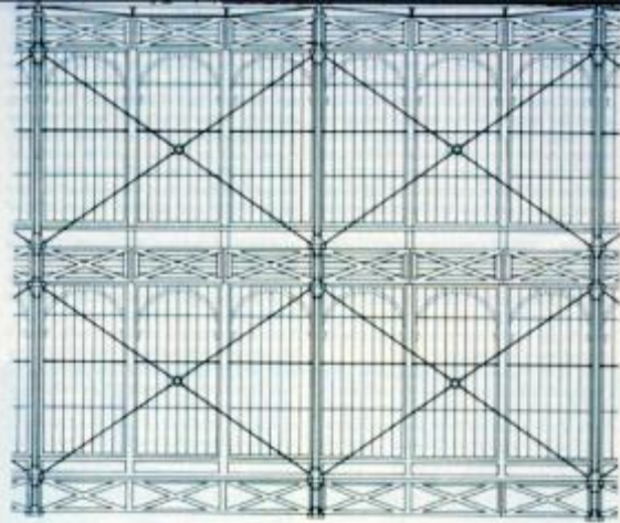
WROUGHT-IRON RODS provided a rigid support for the exterior walls of the Crystal Palace, which had no internal walls to stiffen it. Visible from inside and out (the interior view is shown here), these cross braces added to the building's strikingly contemporary appearance.
