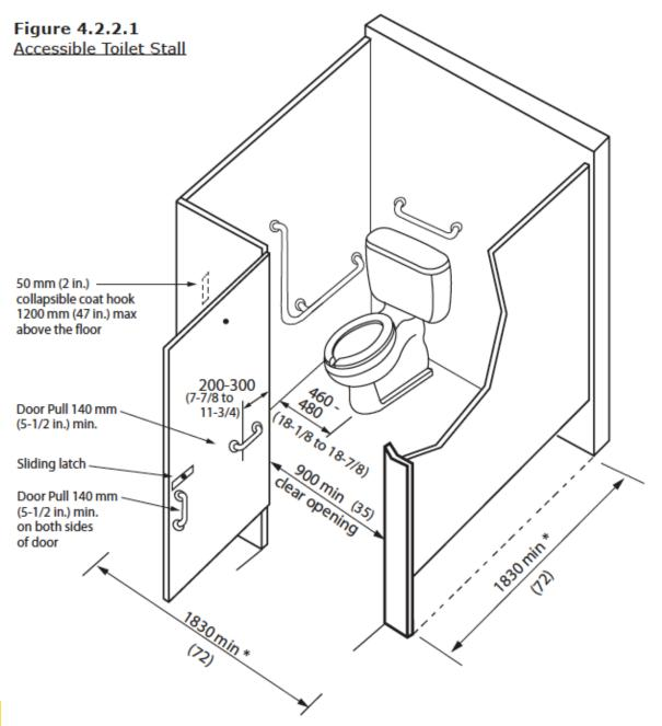
NOTE: In a retrofit situation where it is technically infeasible to provide the required clearances, the dimensions marked with an \* may be reduced. Refer to 4.2.2 - Design Requirements.
