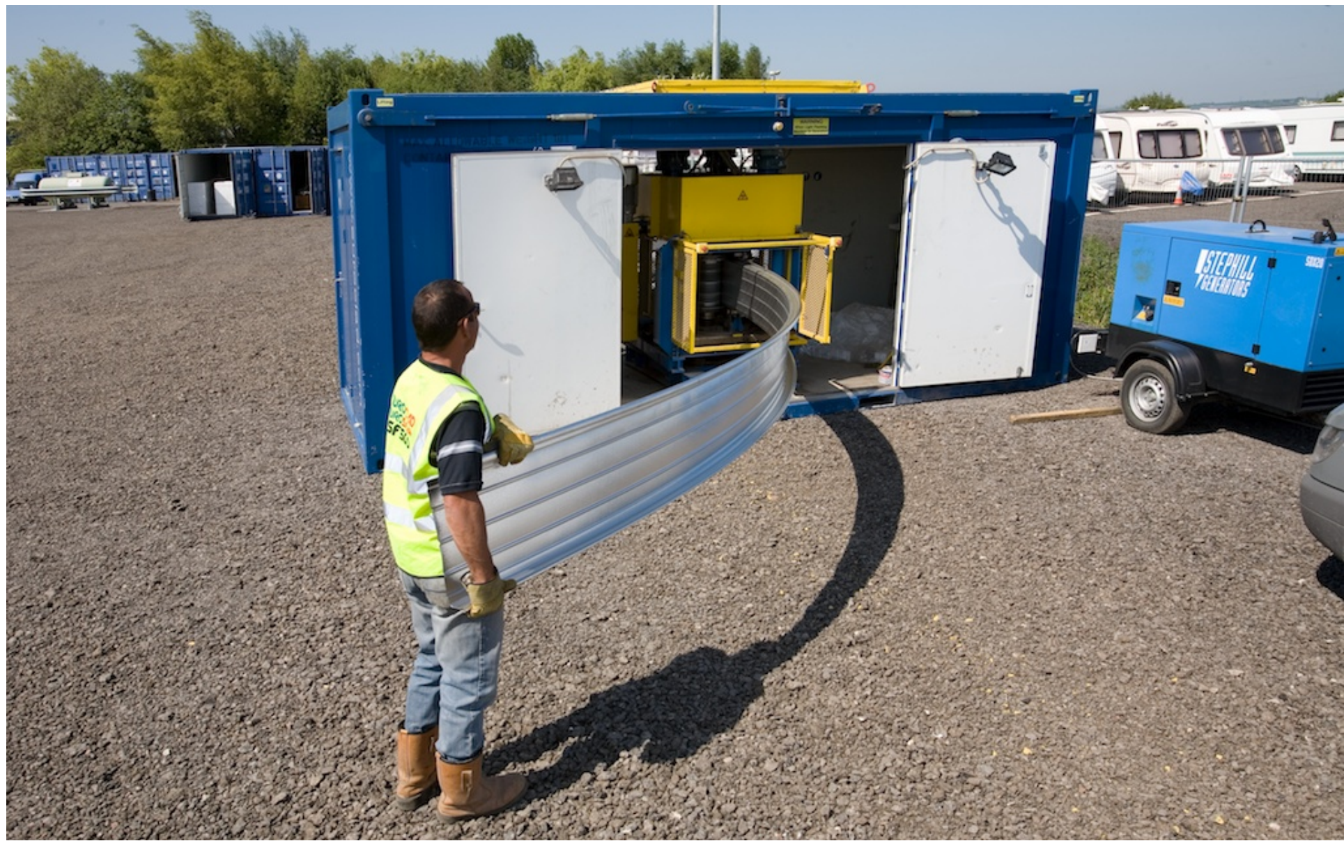
The long panels can be curved on site to fit onto curved roofs.
