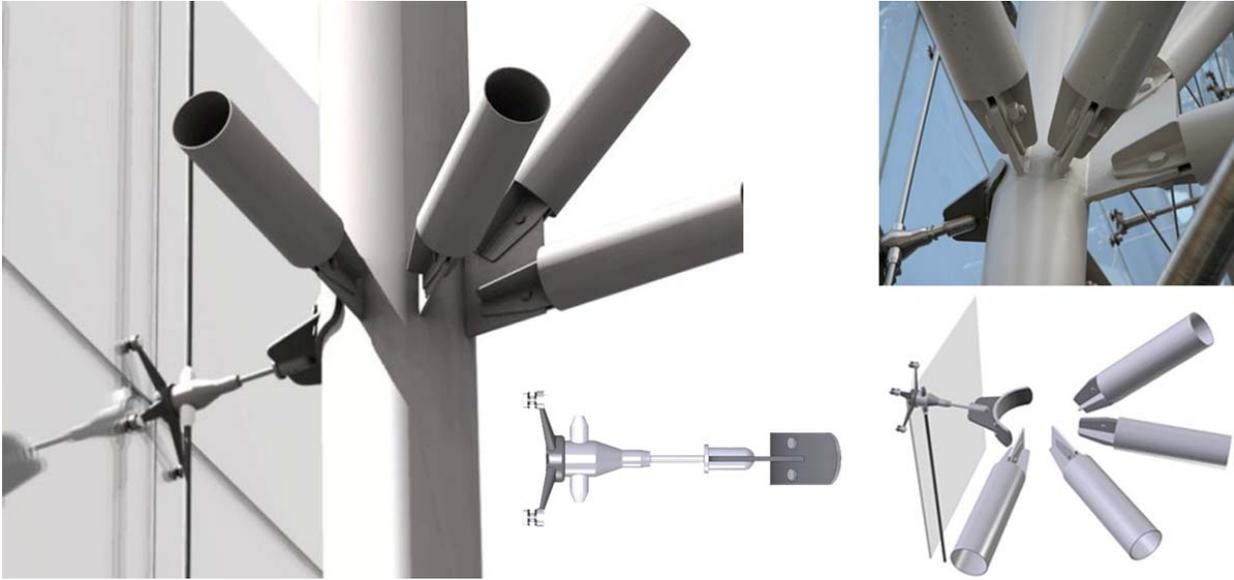
Figure 2. A detail from Polshak Partnership's Rose Center (original photo in top right) explored in different manners through an interactive 3D PDF model
