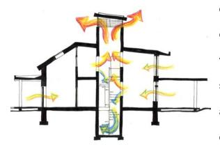
operable windows in the building envelope and travels into the central ventilation shaft. Inside the shaft, the stack effect occurs with warm air rising and exiting the building, and cool air dropping to the food storage area
