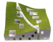
that the swooping green roof was not only added a level of aesthetic complexity to the project but was completely pragmatic in achieving the goals of design such as creating a vista across one diagonal while maintaining a narrow access way across the other diagonal of the square complex. The roof was an undulating mesh that covered units ranging from two levels to 3.5 levels high with varying square footages to accommodate programmatic requirements. (NL Architects, 2002).
