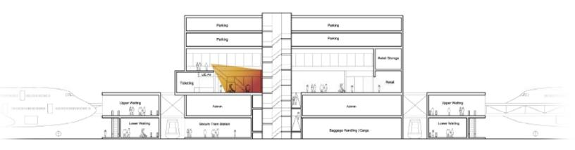
We designed our airport using with the principles of theatre in mind. In section, the mezzanine level serves as an observation deck to the security entrance and the main mall corridor, the largest non-secure area of the airport. The mezzanine is filled with long-term uses, such as restaurants and cafes.
