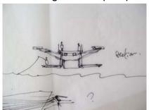
A series of investigations through sketches and models helped create the foundation for the final bridge form. From the initial sketches, the intention was that for the pedestrians to be able to utilize the bridge as an open space, with two or more levels that would enable flexibility in program and circulation. One possibility was to create a single pedestrian deck and another below
