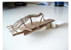
possibly and drape them over steel pylons that point out at each end. The cables are then pulled over and secured to concrete foundations that are placed in the landscape. At the same time, the concrete base supports two parallel steel box girders that support in addition to the suspension cables. At regular intervals, steel U frames are positioned to bear the weight of the bridge and transfer it onto the cables. The U
