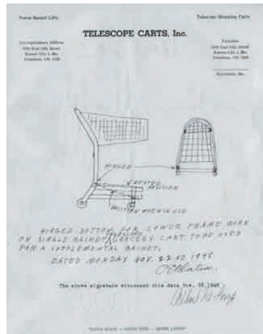
[4] original drawing of a telescope cart by inventor orla e. watson image © archives center, national museum of american history, behring center, smithsonian institution
