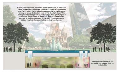
In order to create an unusual and bright underground world under Copley Square, 70-foot wide strips of reflecting pools would be infused with glass lenses just under the surface of the water. These would let bright daylight, magnified by the water, ripple along the pathways. Heated in the winter to avoid snow and ice build up, each lens would acts as an underwater skylight.
