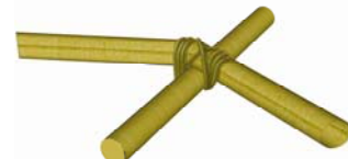
Figure E. Typical rope-and-peg connection used in the Tree Pod.
