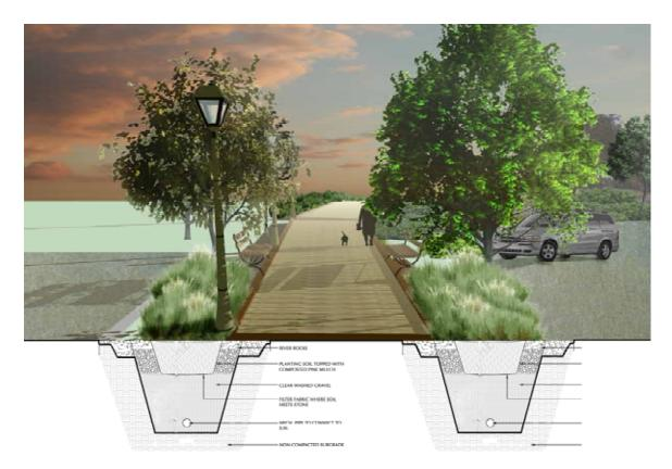
realized how valuable they could be for the filtration of run-off water. Parking was a component of the design, and I wanted to make sure that the runoff from these areas was correctly treated. I can see how valuable these would be in even larger applications.
