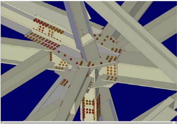
Figure : A single connection isolated in X-Steel
