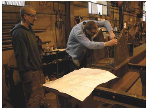
Figure 6: A drawing using standard orthographic projections sits aside the steel whose accuracy is checked with a carpenter's square, pencil and tape measure.
