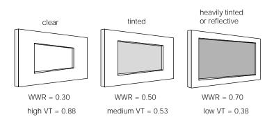
Effective Aperture (EA) is visible transmittance (VT) x window-to-wall ratio (WWR). These three windows all have the same EA.
