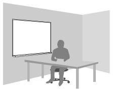
The most comfortable seating is with the window to the side—task is well illuminated and the source is not in direct line of sight.
