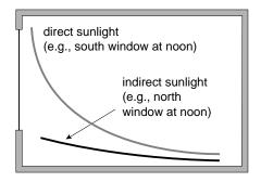
Curves show light levels when a window is facing the part of the sky that has the sun versus the sky away from the sun (daylight only, no direct beam in the room).
