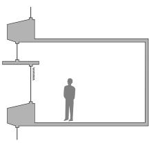
Deep wall section provides self-shading, allows easy integration of light shelf, creates surfaces that mitigate glare, and reduces noise transmission. Sloped surfaces also help soften glare.
