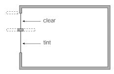
Different apertures for daylight and view: clear glazing above for maximum daylight, tinted glazing below for glare control. The structure between the two provides a visual break and an opportunity to attach a light shelf or shading device.
