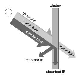
An ideal spectrally selective glazing admits only the part of the sun's energy that is useful for daylighting.
