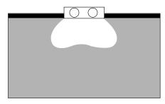
Direct lighting, typical candlepower distribution from ceiling-mounted luminaire
