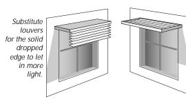
Use louvers in place of solid overhang for more diffuse light while still shading.
