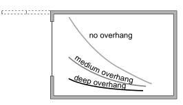
The curves indicate light levels. Overhangs reduce light and glare near the window, creating a softer gradient in the room.
