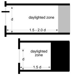
A rule of thumb for daylight penetration with typical depth and ceiling height is 1.5 times head height for standard windows, 1.5 to 2.0 times head height with light shelf, for southfacing windows under direct sunlight.
