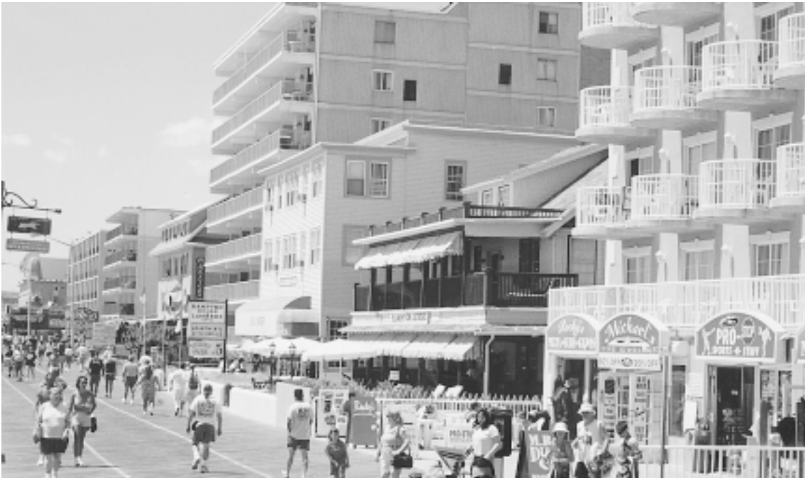
Fig. 3 Balconies Buildings in this summer resort use many kinds of balconies to reduce the cooling load and to provide pleasant space for occupants. These buildings face the ocean toward the east, so the balconies are effective for controlling sunlight mainly around the middle of the day.
