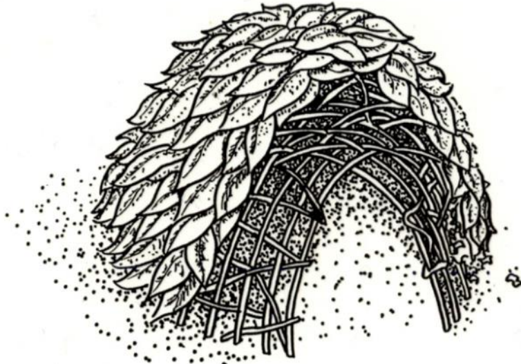
Figure 3.27: Simple dome hut of Banbuti Pygmies is a woven frame of twigs covered with large leaves. (Redrawn from "Primitive architecture and climate," by Fitch and Branch. Copyright © 1960 by Scientific American, Inc. All rights reserved.)
